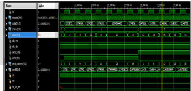
Fig. 5. Simulation results of ATC Disable logic
